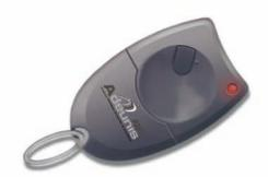
ARF7565 remote controls are 868.3MHz ASK unidirectional remote controls that can be decoded by receivers in the ARF6751 range. When transmitting, the remote controls transmit a command protocol complying with the NF S32-002 (§9.2.2)
