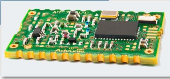
High-performance, long-range radio module with embedded **M-Bus** protocol, for data exchange in stationary and mobile systems between gas, water, heat, electricity meters and concentrators.
